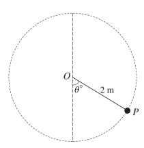
A particle P of mass 0.4 kg is attached to one end of a light inextensible string of length 2 m. The other end of the string is attached to a fixed point O. With the string taut the particle is travelling in a circular path in a vertical plane. The angle between the string and the downward vertical is  $\theta^{\circ}$  (see diagram). When  $\theta = 0$  the speed of P is 7 m s<sup>-1</sup>.
